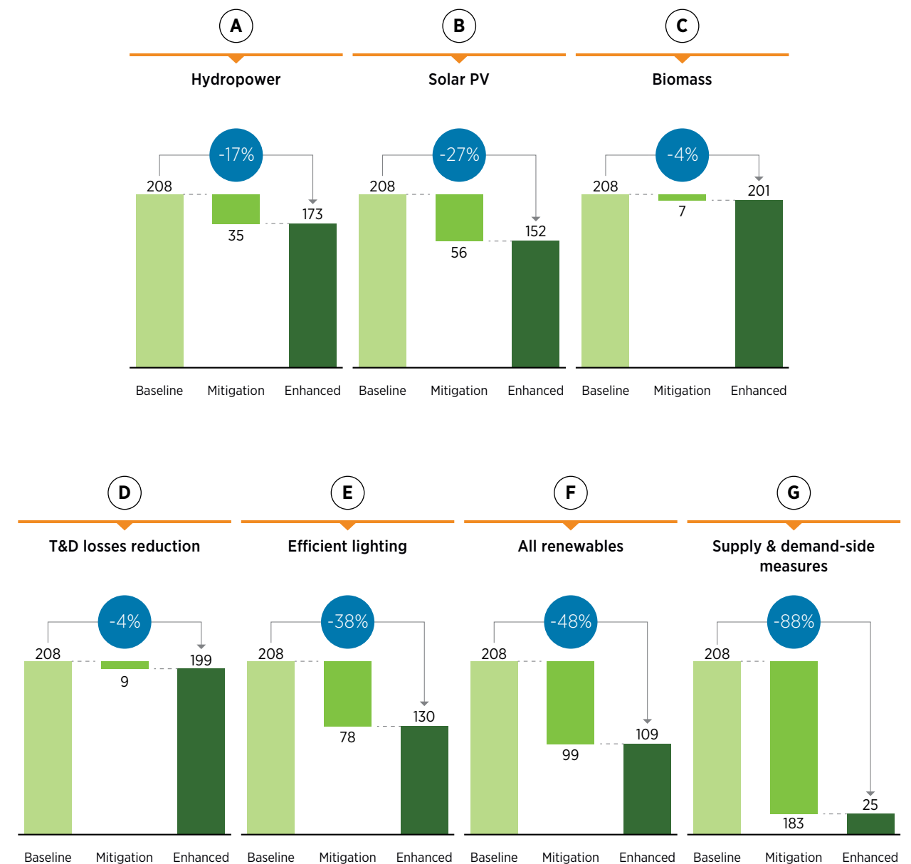
Figure S1 GHG emissions reductions potential of power sector mitigation options by 2030 (% , ktCO 2 )*
